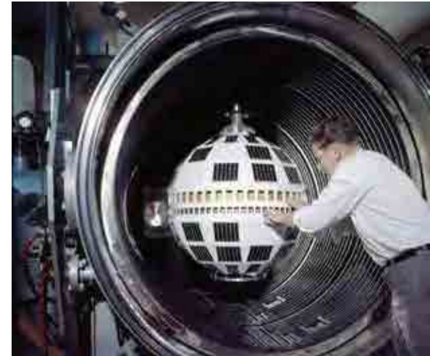
Thermo Vacuum Chamber Test to Determine Thermal Effects of Sunlight (1962) Photo courtesy AT&T Archives and History Center
