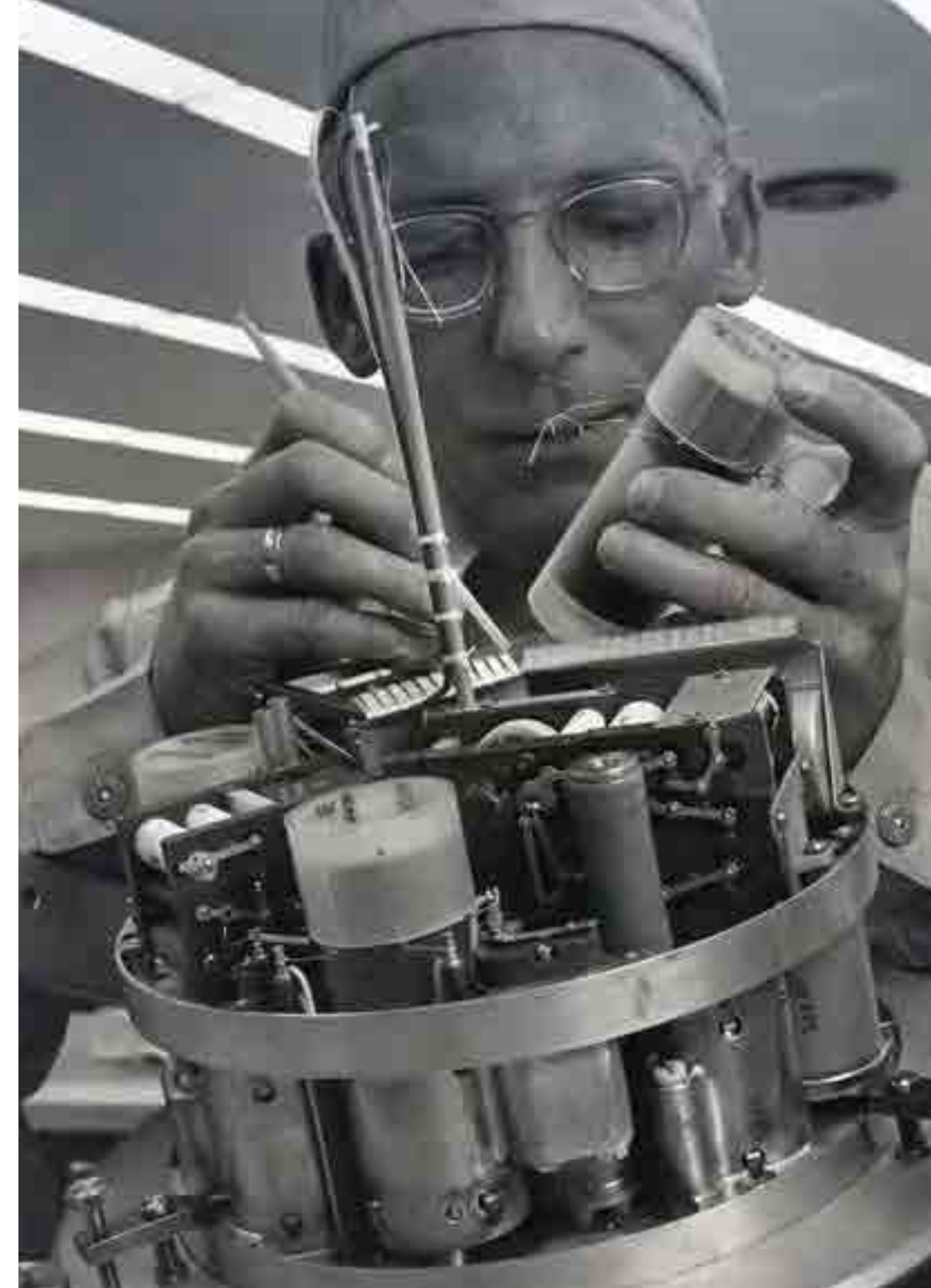
Manufacturing an Undersea Repeater, Clark, NJ Plant (1962) Photo courtesy AT&T Archives and History Center
