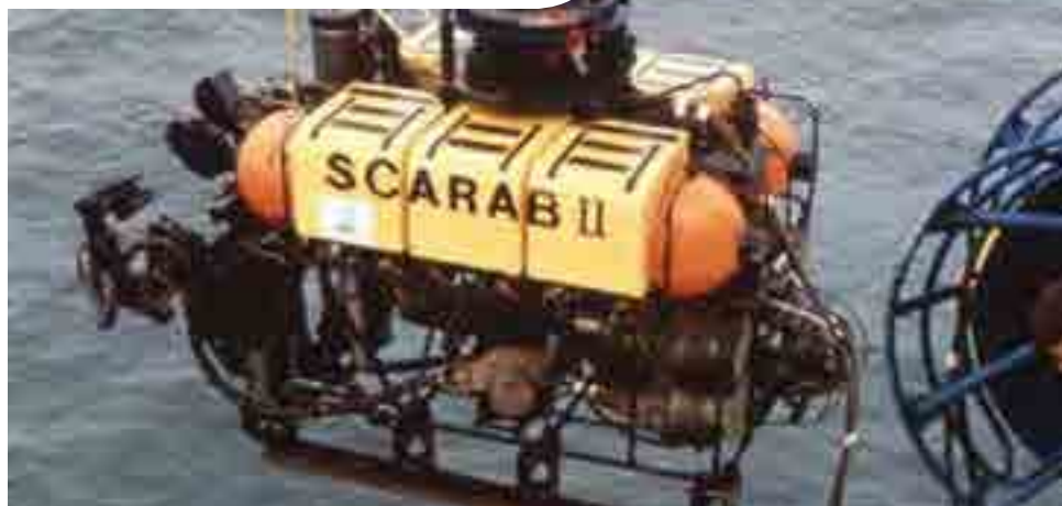
AT&T SCARAB, Remote Controlled Cable Repair Submarine (1986) Photo courtesy AT&T Archives and History Center
