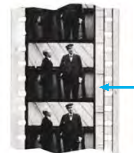
A section of sound film showing the photographic recording. The arrow points to the sound track.
